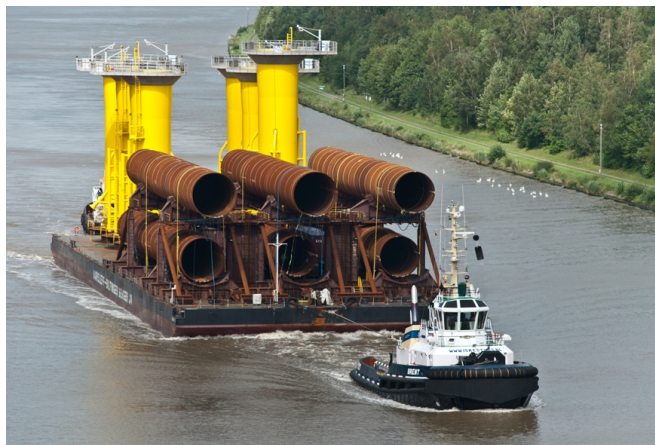
Figure 1.6: Monopiles and transition pieces towed to site on a barge (ISKES (2016)).
