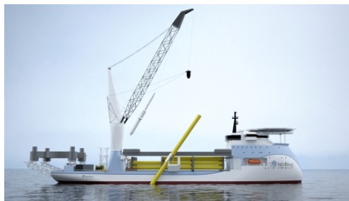
Figure 1.9: NorWind offshore wind foundation installation vessel and Knud E. Hansen upending trolley (OffshoreWind.biz (2011), K.E. Hansen A/S).
