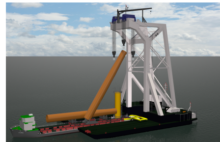
Figure 1.9: NorWind offshore wind foundation installation vessel and Knud E. Hansen upending trolley (OffshoreWind.biz (2011), K.E. Hansen A/S).
