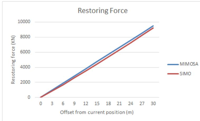
Figure 5.5: Restoring force curve from MIMOSA and SIMO
