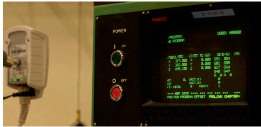
Fig. 3. Camera observing NC machine
