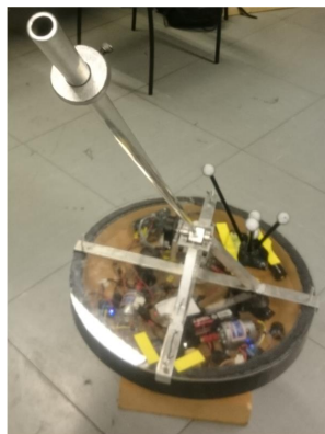
(a) Additional weight added to the top of the pendulum.
