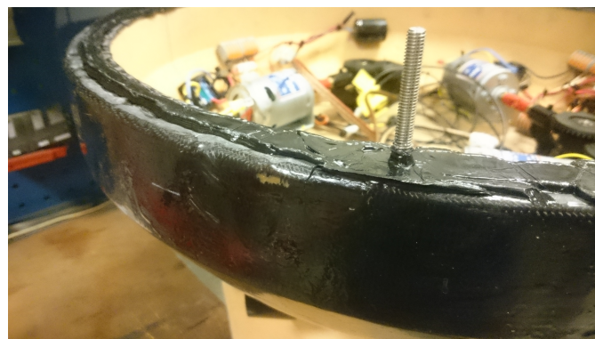
Figure 2.18: Seal to waterproof the vessel.
