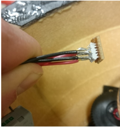
(a) One of several soldering points with high risk of short circuit due to lacking heat shrink tube.
