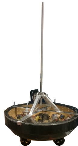
(b) Pendulum fitted to the CS Saucer. The pendulum is longer than in the picture.
