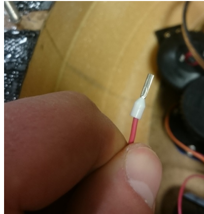
(b) Termination sleeve fitted to the wire end to ensure safe and durable termination.
