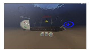
Figure 1.6: A proposed way to use augmented reality to help the user during ROV operations. (Juan & Sanz 2015).
