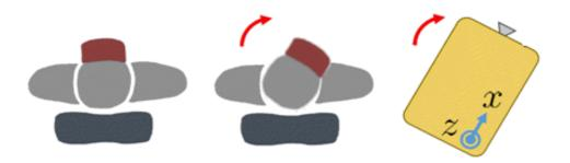
Figure 4.2: The proposed head movements giving yaw command to the ROV. In the figure a clockwise rotation of the head in yaw give a clockwise motion around the z axis for the ROV. Figure from (ChangSu Ha & Lee 2015).
