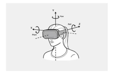
Figure 2.2: The OR can measure all six degrees of freedom. This is the way the translations and rotations is defined in the OR software.
