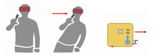
Figure 4.4: The proposed head movements giving sway command to the ROV. A movement in positive y-direction with the head gives a movement for the ROV in positive y-direction. Figure form (ChangSu Ha & Lee 2015).
