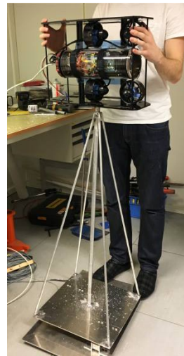
(b) ROV setup on rig for testing heave forces.
