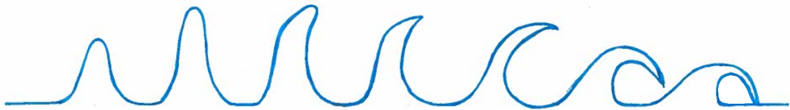
Figure 6.3: Sketch of the development of a plunging breaker.
