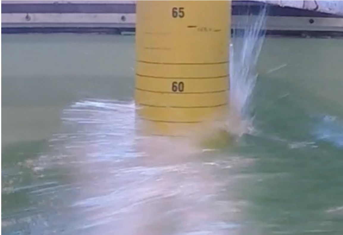
Figure 6.13: Plunging breaker hitting the pile.
