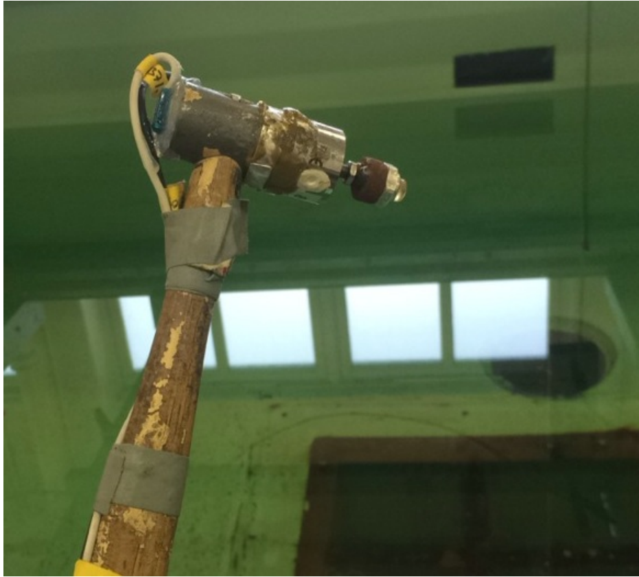
Figure 4.16: Hammer with a load cell in the tip used for static tests.
