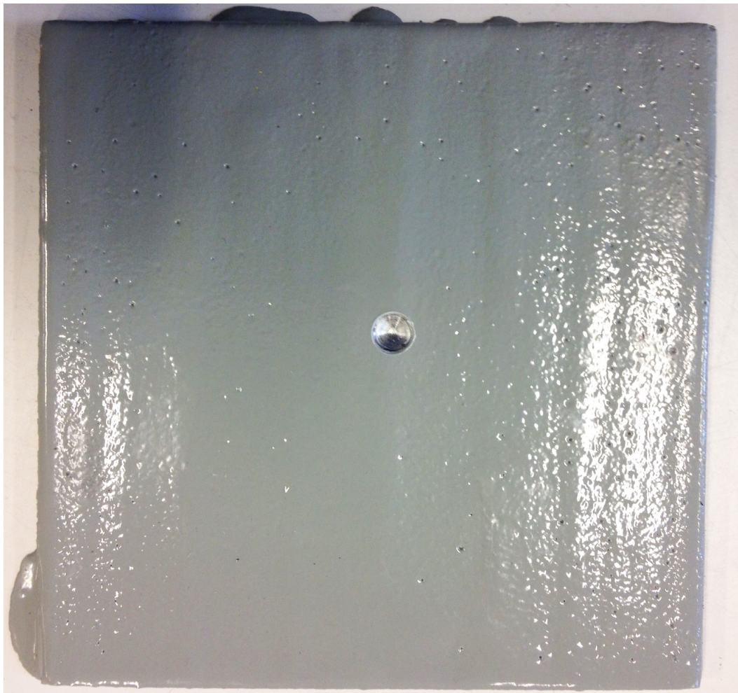
FIGURE 19 TSA WITH EPOXY COATING AND COATING AND MANUFACTURED COATING FAILURE.
