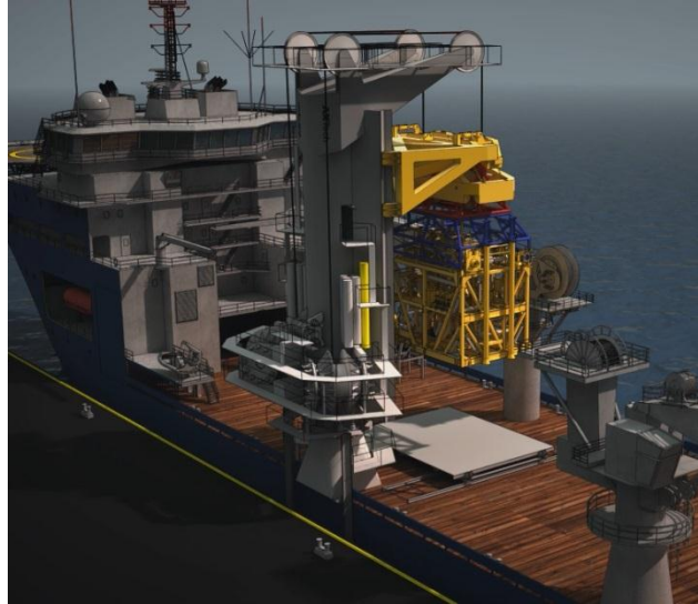
Figure 3 The SHS system attached to North Sea Giant (Source: (Tecnip_Aagard_B_Final, 2012))
