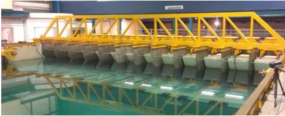
Figure 16 The wave generator at Oceanide
