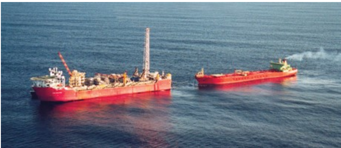
Figure 5.1: Ships during tandem offloading (SOFEC (2016))
