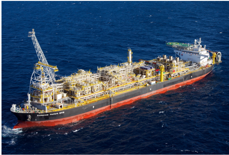
Figure 1.1: A typical FPSO ( Modec (2015) )
