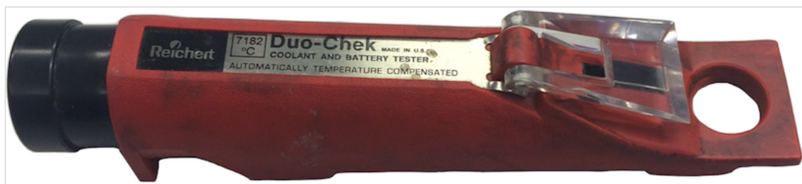
Figure 9.3: Handheld refractometer used to determine the PG concentration.
