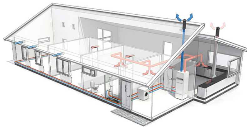
Figure 3.2: Illustration of an exhaust air/water system [5].
