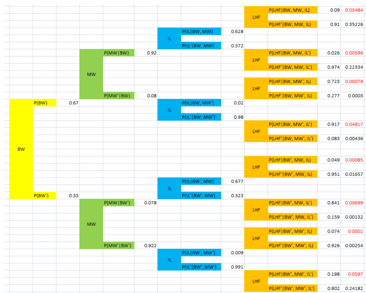
Figure 15: Influence diagram converted to event tree for loss of head and pressure (LHP)
