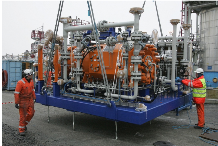
Figure 26: Subsea compressor for Åsgard at K-lab, source http://www.statoil.com/
