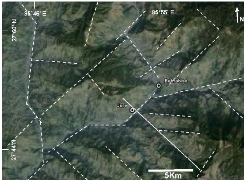
Figure 2.9: Major lineaments (dashed lines) near the rockslide area. The most prominent lineament in NW-SE direction is through the landslide zone (solid line) (Champati Ray and Chatteraj, 2014).
