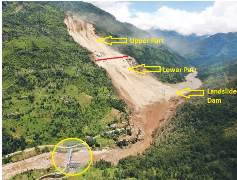
Figure 2.6: Jure landslide components with landslide dam. The red line is the resistant layer dividing the upper and the lower part. The intake of Sunkoshi Hydropower Project is shown in the yellow circle (Modified from KathmanduPost (2014))
