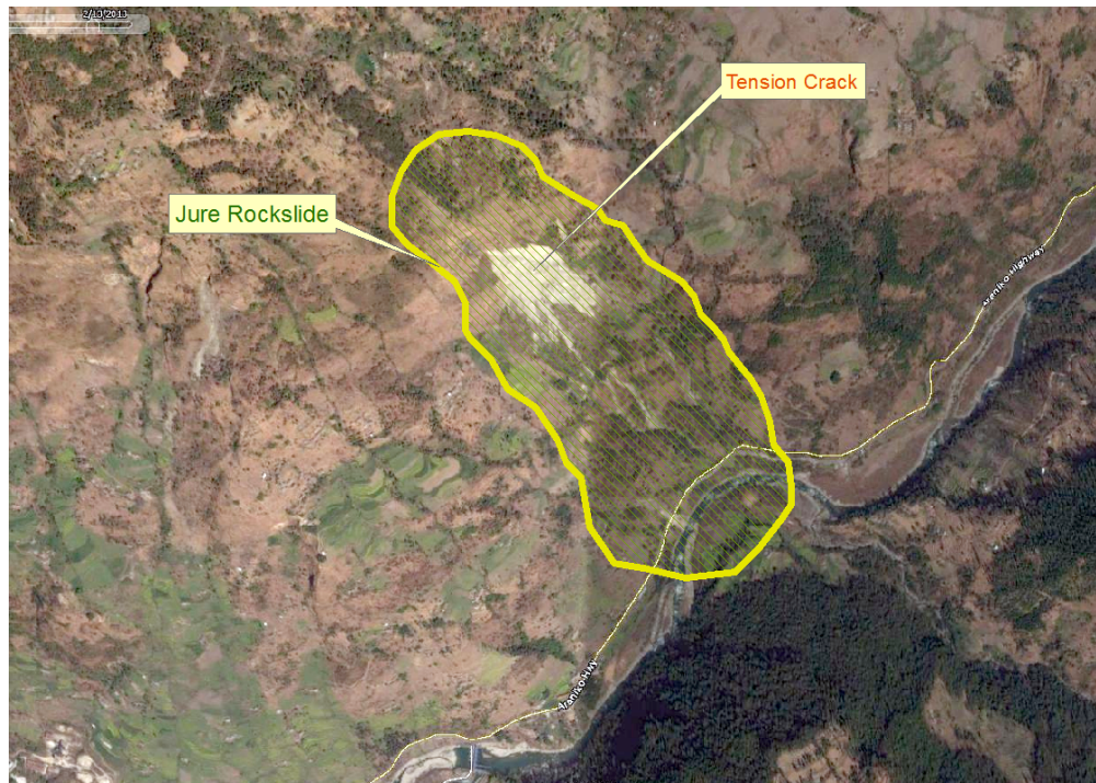
Figure 2.7: Tension cracks seen in Jure rockslide as of 13 th of February 2013. Modified from GoogleEarth (2016) historical archives.
