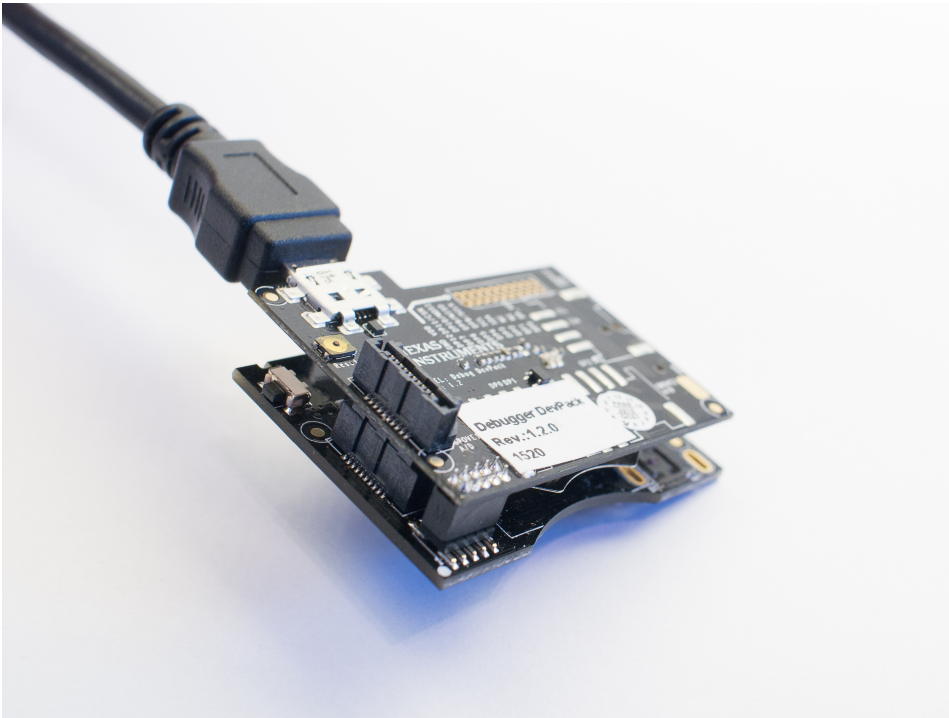
Figure 4.3: Debugger DevPack connected to SensorTag
