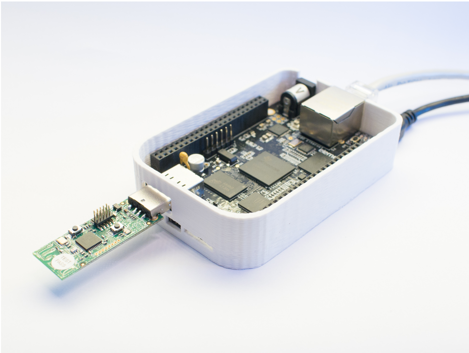
Figure 4.4: Border Router made of Beagle Bone Black and CC2531 radio module
