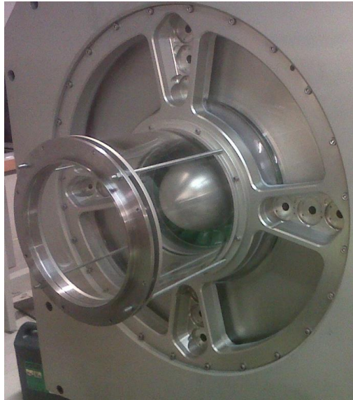
Fig. 18: Plexiglas windows for flow visualization
