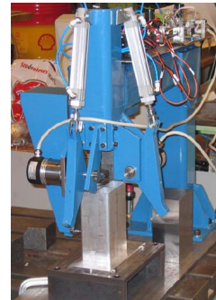
Figure 2: Laboratory version of the complete welding jig with one work piece in position ready for clamping.
