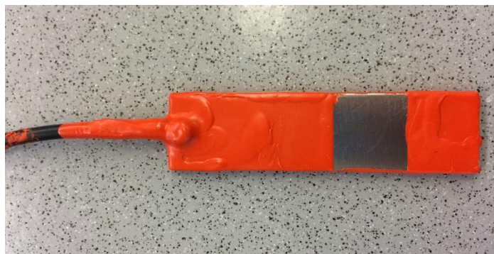
Figure 3.2. Steel sample coated with Micro Super XP 2000 Stop-Off Lacquer.
