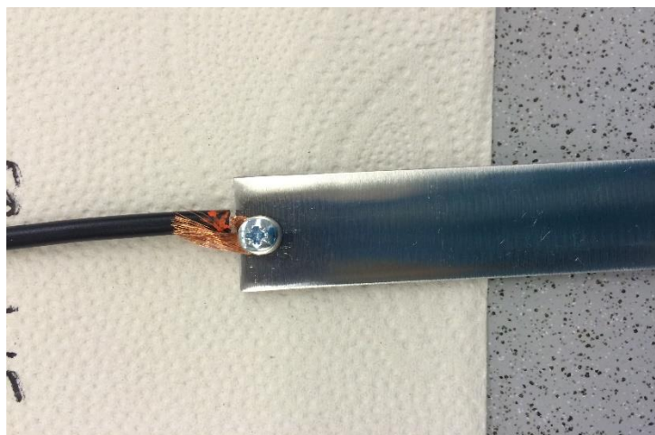
Figure 3.3. Connection of wire to metal sample. The insulation on one end of a banana plug wire is stripped off and forced in contact with the sample with a screw and a washer.
