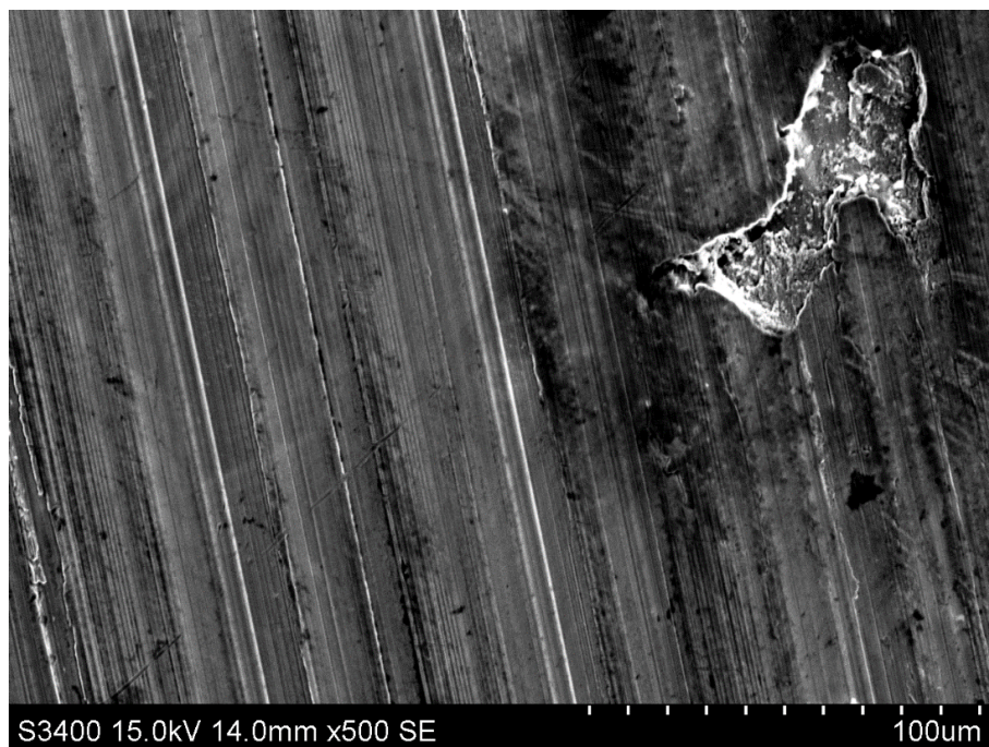
Figure B.4. SEM image of an X65 CS sample from galvanic corrosion testing between X65 CS and AlZnIn in NaCl. The image was taken prior to chemical cleaning.
