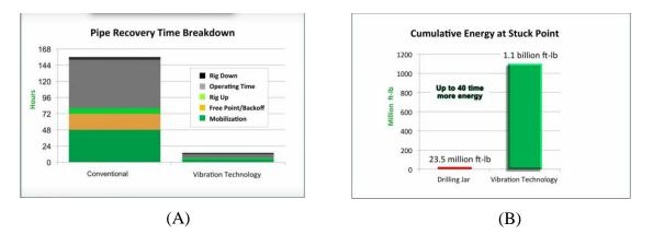
Figure A.2 Charts highlighting the benefits of resonant vibration for releasing stuck pipe compared to conventional method with regards to recovery time and actual energy transferred to the stuck point (Layne, 2015).
