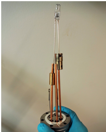
Figure 4.1.: Evaporator for powder compounds. Current is run through the bulb leading to heating of the powder. Subsequently evaporation occurs. The evaporation is primarily controlled by varying the current.
