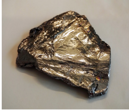
Figure 4.2.: Natural molybdenite crystal used as a substrate for doing the experiments.
