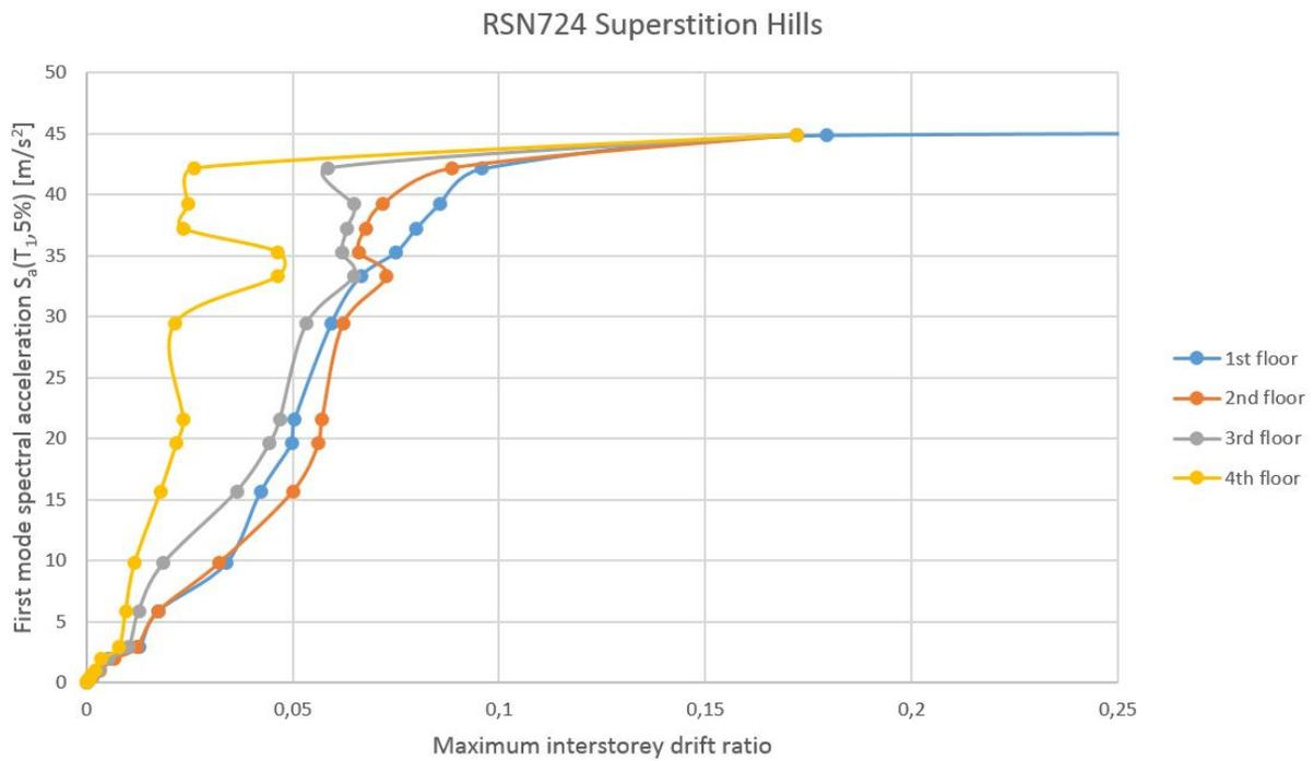
Figure 8.12: IDA curves showing maximum interstorey drift ratio for each floor, for the RSN724 record
