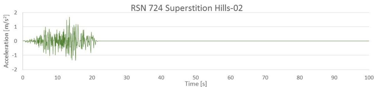
Figure 6.10: RSN724 Scaled ground motion time-history
