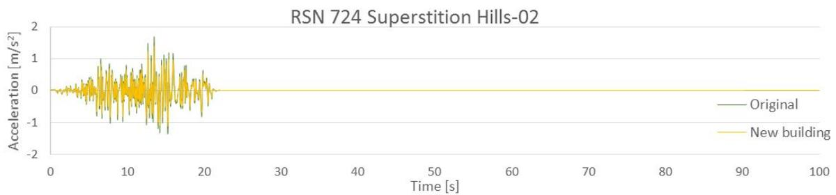
Figure 9.3: RSN724 Scaled ground motion time-history
