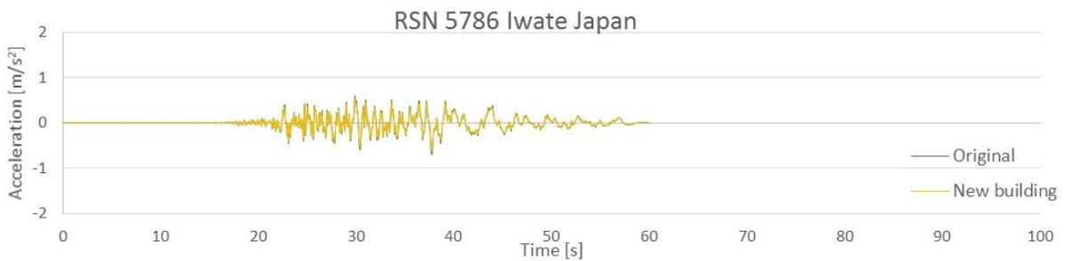
Figure 9.7: RSN5786 Scaled ground motion time-history
