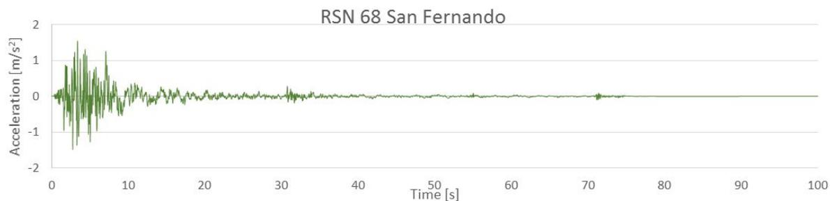
Figure 6.8: RSN68 Scaled ground motion time-history
