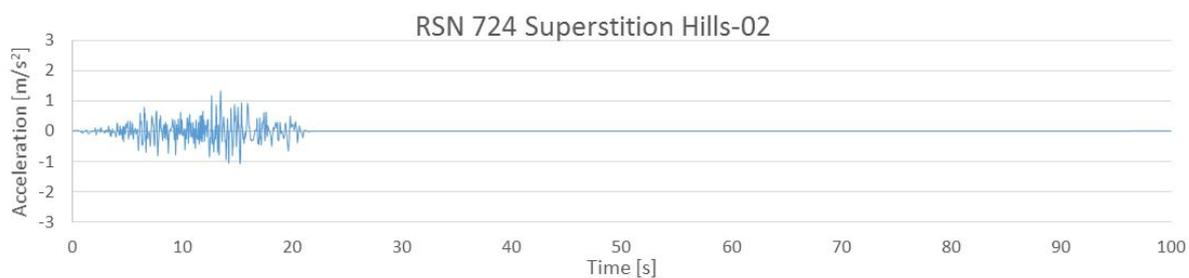
Figure 6.3: RSN724 Unscaled ground motion time-history
