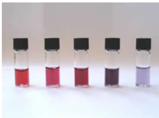
Figure 2.4: Gold nanoparticles of different sizes (4 to 80 nm from left to right) suspended in water, showing different colours. 2
