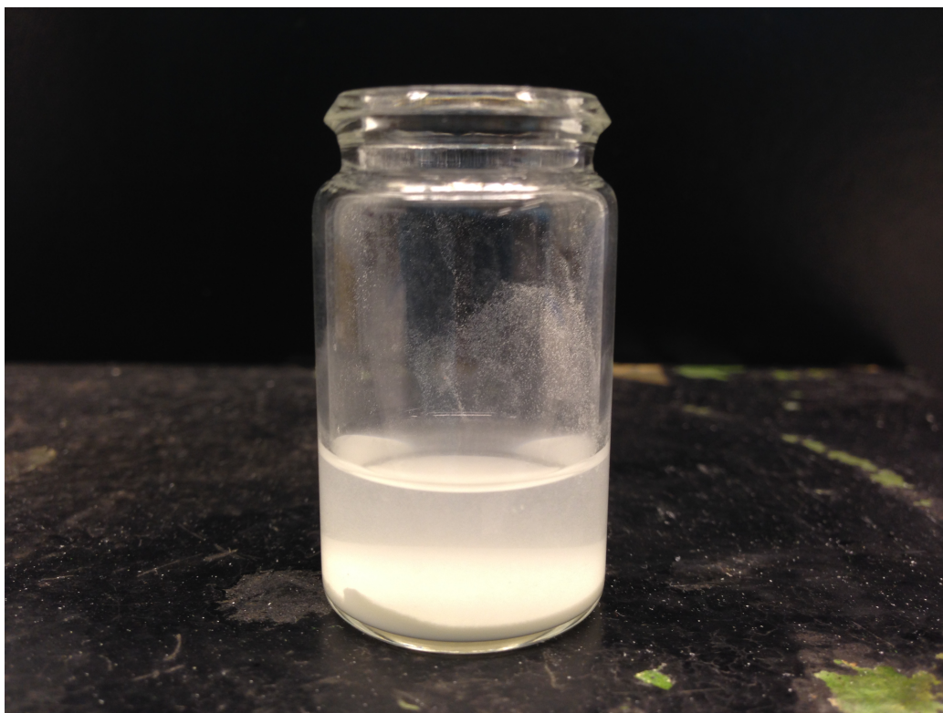
Figure 4.16: 10:1-15min mixed with diethyl ether showing sediments and large flocs.
