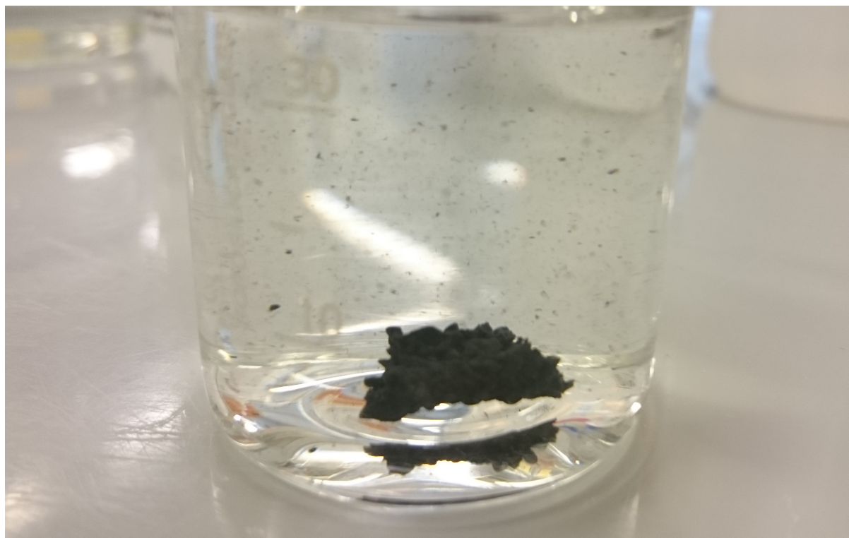
Figure 4.2: The failed attempt at testing the stability of the hexagonal phase of nanocrystalline \text{YTi}_{0.15}\text{Mn}_{0.85}\text{O}_{3\pm\delta} in alkaline conditions. Particles of carbon tape can be seen floating around in the DI water.
