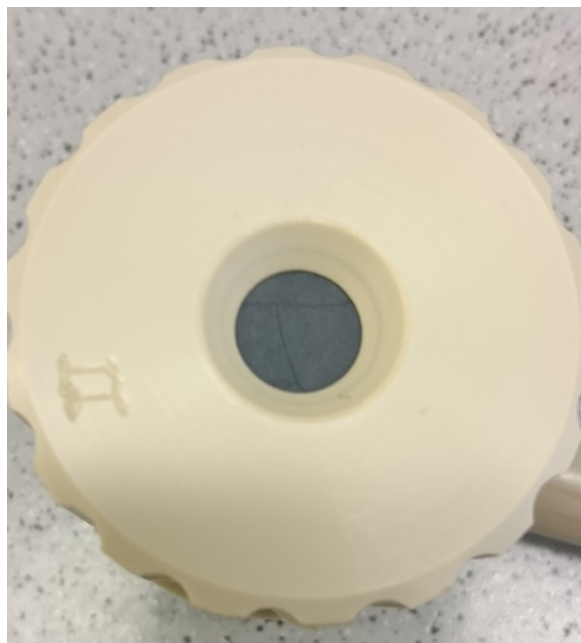
(a) When tightening the teflon casket on the flat specimen electrode, the pressure on the disc caused it to fracture.
