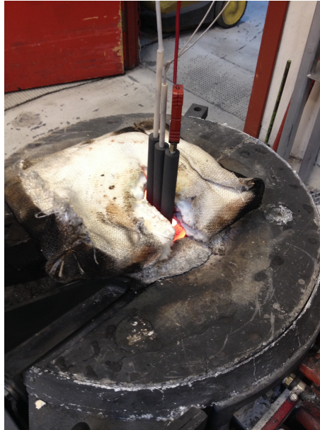
Figure 3.7: The crucible placed in the furnace to measure the radial temperature gradient. There were three measuring points from the crucible wall to the center of the crucible. The opening in the furnace where the crucible is placed is 18 cm in diameter.
