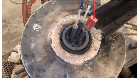
Figure 3.4: Set up for comparison of C-thermocouples and S-thermocouple at 1500 °C. The opening in the furnace has a diameter of 18 cm, and the crucible has an inner diameter of 11 cm.
