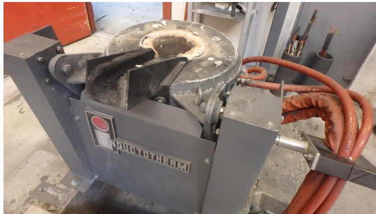
Figure 3.1: The induction furnace used for the experiments. A carbon crucible fits in the furnace opening, which is 18 cm.
