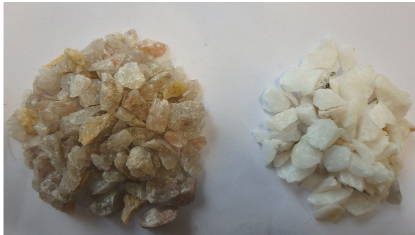
Figure 2.5: Two types of quartz. The one to the left has a higher impurity content. The photo is taken by the author for use in this thesis.
