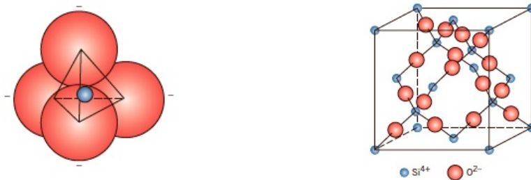
(a) Silicon-oxygen tetrahedron, \text{SiO}_4^{-4} . (b) The arrangement of silicon and oxygen in a unit cell of cristobalite [17] .
