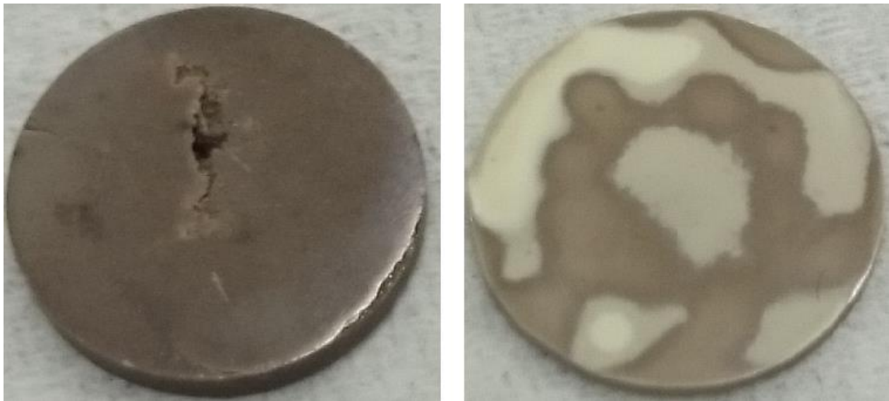
Figure 4.7: Pictures of a sintered BTO-c sample (left) and sintered BTO-n sample (right) 14 days after sintering. Both samples were sintered at 1300 °C for 4 hours.
