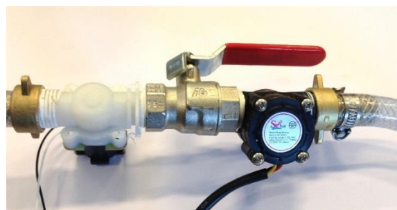
Figure 5.19 Solenoid valve and flowmeter attached to water supply
