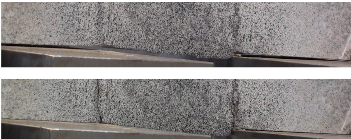
Figure 4.13: Mounting of test sample II before (over) and after (below) the shear test.
