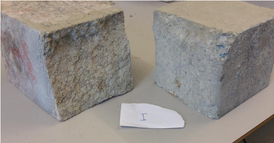
Side one of test specimen I after failure:
