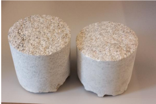
Figure 4.1: Example of drilled core samples
