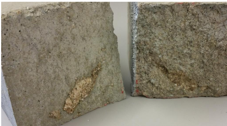
Figure 4.12: Rock defect in shear test I
