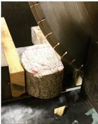
Figure 4.2: Cutting the core samples into cubes
