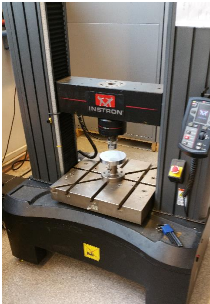
Figure 4.4: The electromechanical testing rig.
