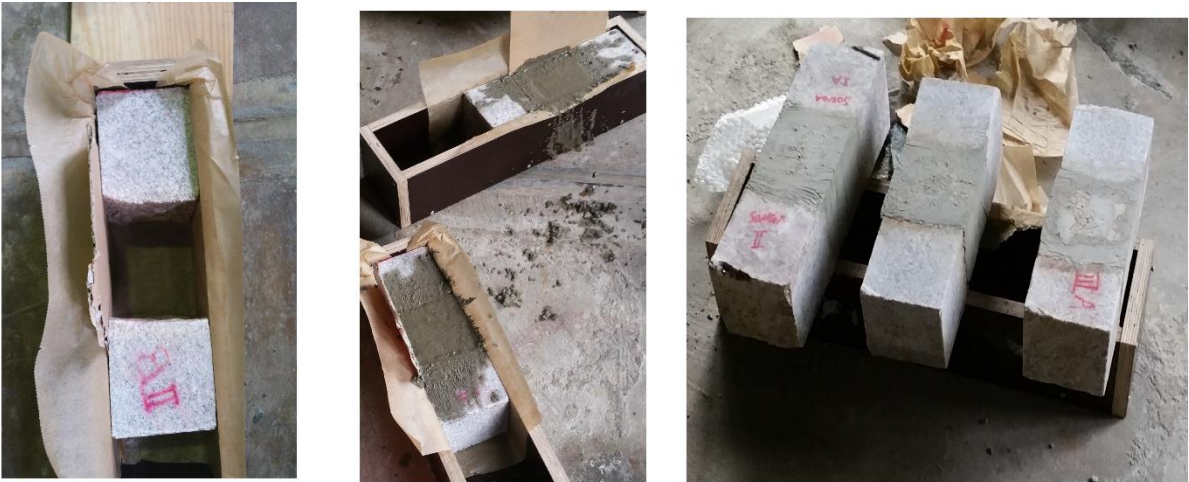
Figure 4.3: Casting of test samples
