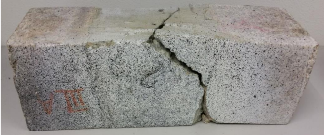
Figure 4.11: Test sample III after failure.
