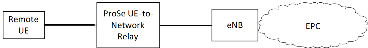
Figure 4.7: Architecture model using a ProSe UE-to-Network Relay
