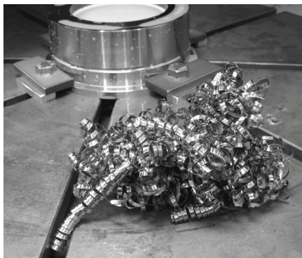
Figure 7: Tangling of continuous chips.
