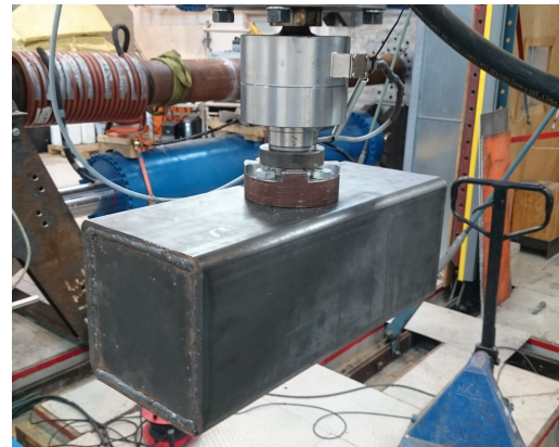
(b) The rigid intruder mounted on a self-made interface between the load cell and the mast.
