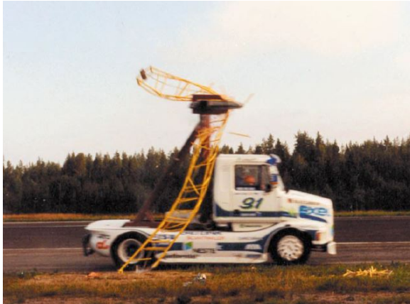
(a) Dynamic impact between impactor and mast [3].
