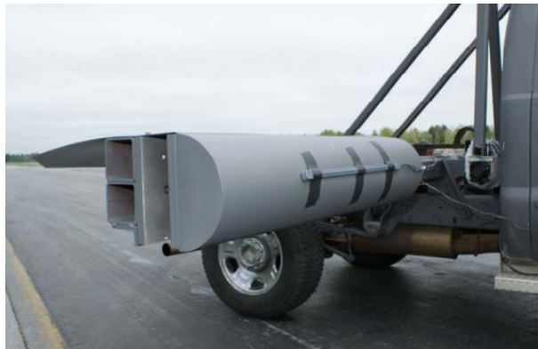
Figure 3.1: Rigid impactor. Photo taken by M.J. Nasad [4] .
