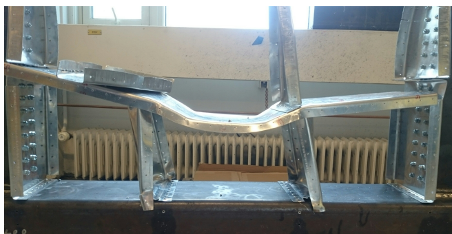
(a) Deformed main-spar after compression test.
