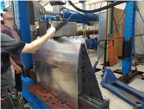
Figure 10 Rigging of soft wing impactor
