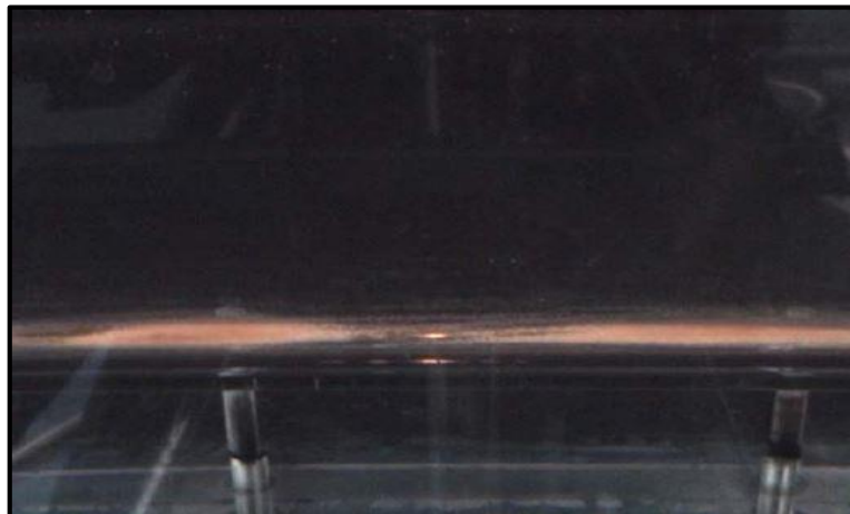
Figure 1.11 Sand dunes at the pipe bottom. Side view. ( C_v=5.38 \cdot 10^{-5} . V_w=0.4 m/s. Yan, 2010)
