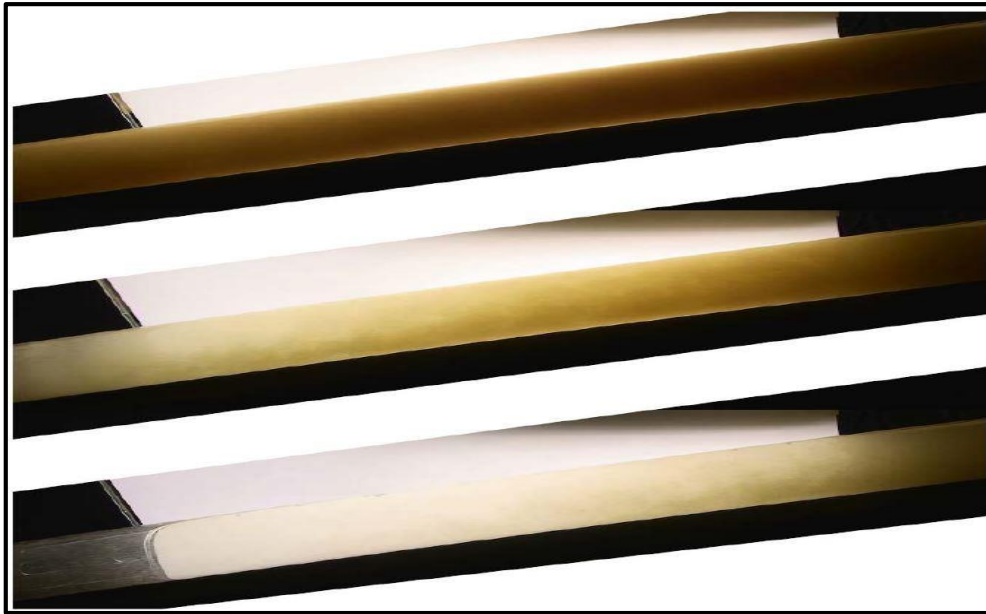
Figure 1.5 Main body and tail propagation of the particle plug (Shabani, 2012)
