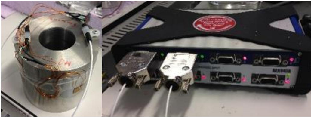
Figure 3.5: Thick walled cylinder with strain gauges and the 8-channel universal amplifier
