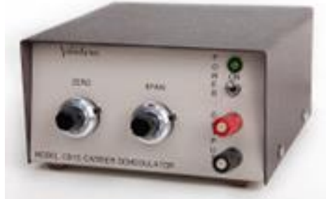
Figure 3.7: The sensor carrier demodulator
