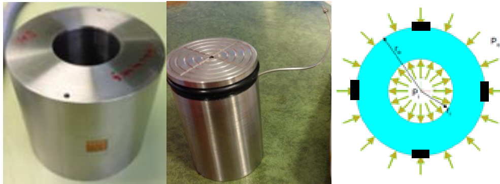
Figure 3.3: Thick walled cylinder, lower piston and a sketch of a thick walled cylinder (Daly, 2003)
