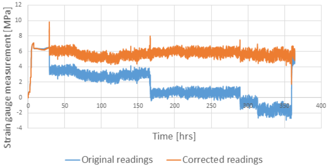
Figure 4.21: Strain gauge measurements of channel 1 of core sample 2
