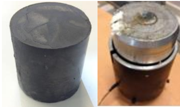
Figure 4.1: The first core sample and salt on top of the loading cell
