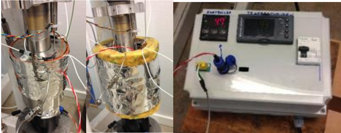
Figure 3.9: The heating element with and without temperature isolation and the control element
