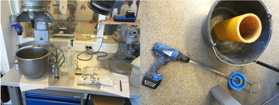
(a) The mixing area with the Hobart mixer. (b) The equipment for the drill-mixing
