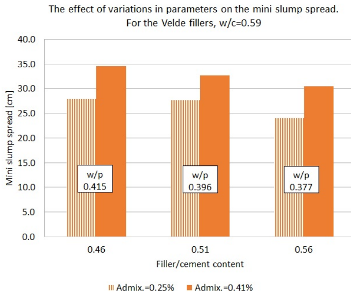
Figure 5.12: How the variation in filler content (filler/cement content), water/powder-ratio and admixture dosage (of total powder content) affect the mini-slump spread in the w/c=0.59 results.
