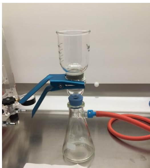
Figure 2.7: The filtration during CWE (Photo: H. Vurucu)
