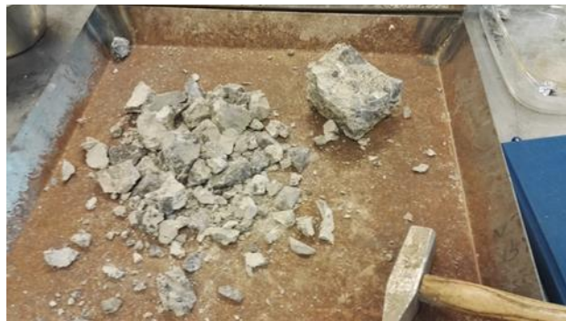
Figure 2.10: Hammering to separate the coarse aggregates from the mortar (Photo: G. Plusquellec)
