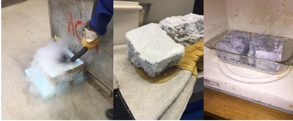
Figure 2.9: The freeze/thaw process using liquid nitrogen and microwave (Photo: H. Vurucu)
