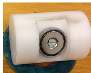
(b) Picture of the piston made of POM (thermoplastic)
