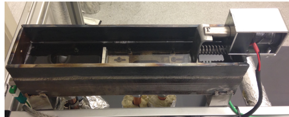
(b) Picture of the solenoid from the side, showing the position of the solenoid and the compression spring. An extra bracket (bended at the top), fixed to the original 90 degree bracket at the right hand side of the thermostat, was providing a connection point for the solenoid. The external end configuration of the plunger was attached with a pin to the bended part of this bracket.
