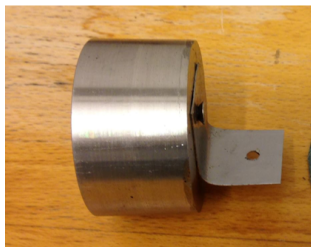
(a) Picture of the piston made of stainless steel
