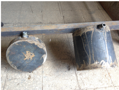
(a) Picture of the application unit to the right and receiver to the left. Connections are welded on to enable attachment to the pipes in the system.
