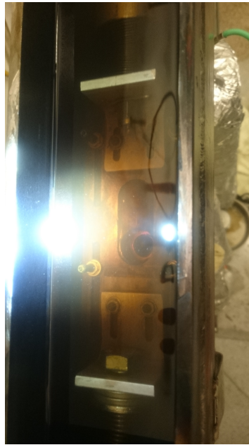
(c) The bellows has expanded to its final position. The liquid inside has reached its boiling temperature, causing vapor formation inside the bellows. The oil entering the thermostat is now leaving through port 3.
