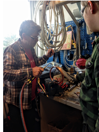
(d) After the coil was cut at the point giving the desired coil laps (approximately 1.5 rounds), the one outlet was closed and soldered completely, whereas the other outlet was soldered to a tube fitting. This tube fitting was then connected to the bellows.
