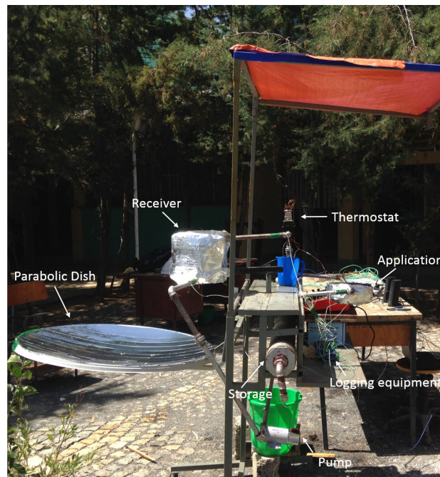
Figure 7.4: Picture of the circulating oil based system setup at Mekelle University. Arrows indicates where the main components in the system are located.
