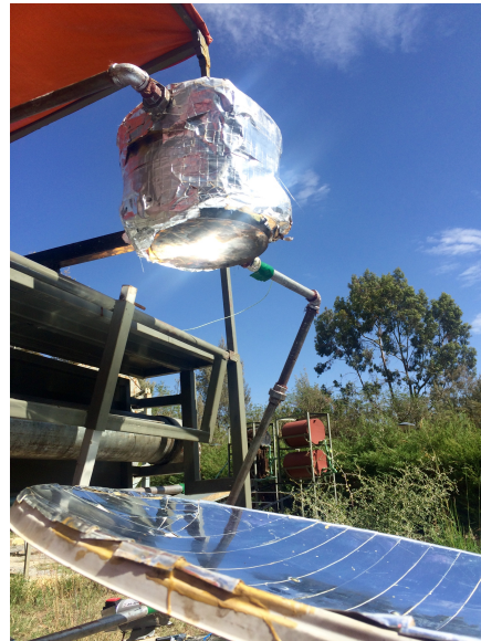
(b) Picture of the offset parabolic dish with the focal point at the receiver.
