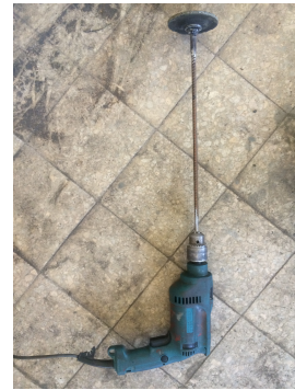
(f) Picture of the grinder attached to the drilling machine.
