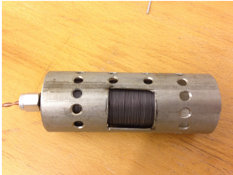
Figure 4.11: Picture of the bellows inside the confining tunnel, after parts of the tunnel has been cutoff. It was believed that this could result in a more efficient overall oil penetration on the surface of the bellows.
