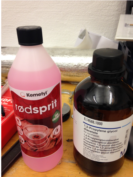
(a) Picture of the ethanol and the 1,2-Propylene glycol diacetate used inside the bellows
