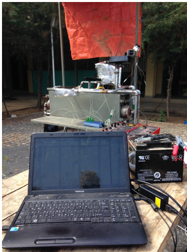
(a) Picture of the computer connected to the data logger, plugged with thermocouples.
