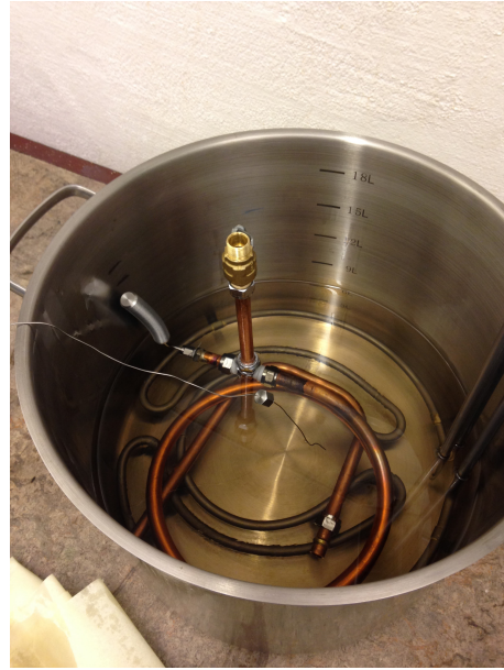
(b) A close-up picture of the gas bellows system. In the picture the heating element can be observed in the bottom section of the oil bath, where the copper coil has been located on top of it (without being in direct contact due to a copper pipe working as a separating unit). A tee-tube-fitting was connected to the outlet of the coil, where the bellows was connected to the one outlet and the valve to the other.
