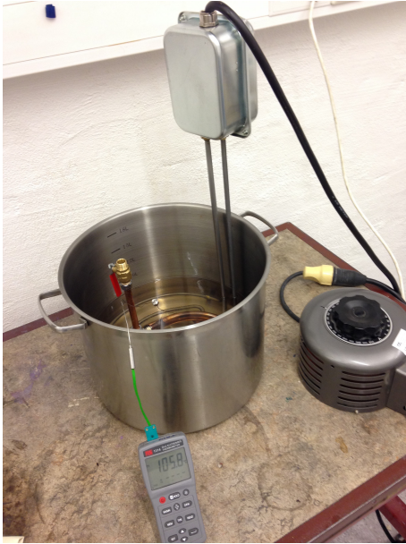
(a) The setup used for the testing of the gas bellows. The oil bath contains a heating element immersed in the oil, together with a copper coil filled with air. The bellows was connected to the coil as visualized in Figure 4.21b. A short copper pipe, connected to the coil, holds the valve which was to be closed at a given oil temperature. The temperature was measured by the temperature reader, and the heat from the heating element was controlled by the regulator.
