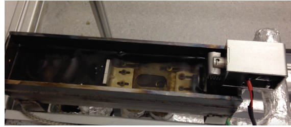
(b) Picture of the solenoid in the latched position.
