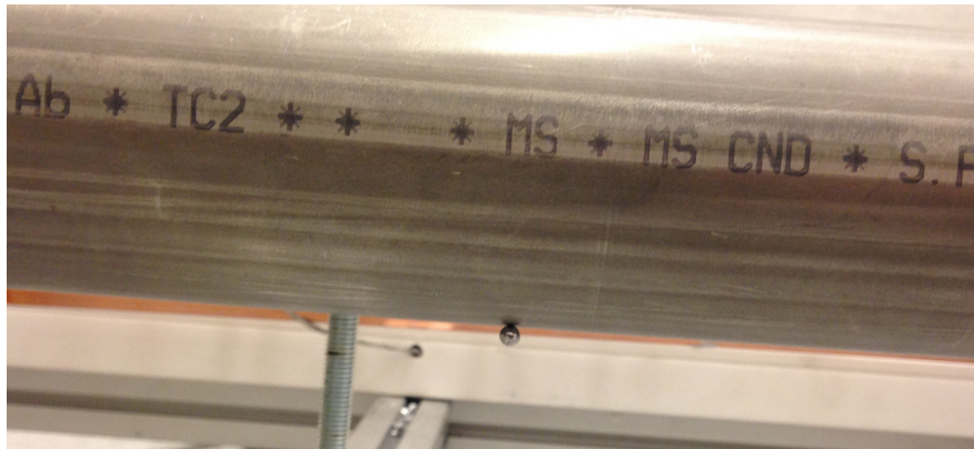
Figure 5.5: The magnet ball travelling on the outside of the storage. At the inside of the storage, at this position, the piston would be located.
