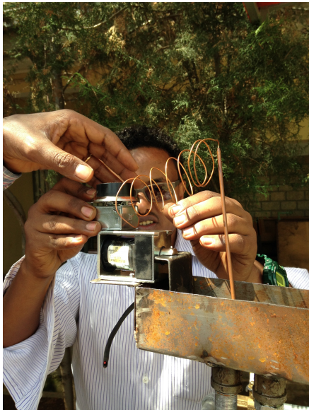
(a) Picture of the thermostat solution with the solenoid and the capillary thermostat.
