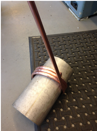
(c) The copper coil made out of 15 mm diameter pipes. The picture was taken right after the coil had been rotated around a cylinder, giving the coil a center diameter of 19.0 cm.
