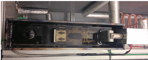
(a) Picture of the solenoid taken from above. Where the bellows once was located, there has been added a supporting stick instead. The supporting stick ensured that only a 15 mm stroke was required (diameter of the ports), and a higher overall pulling force could therefore be obtained.
