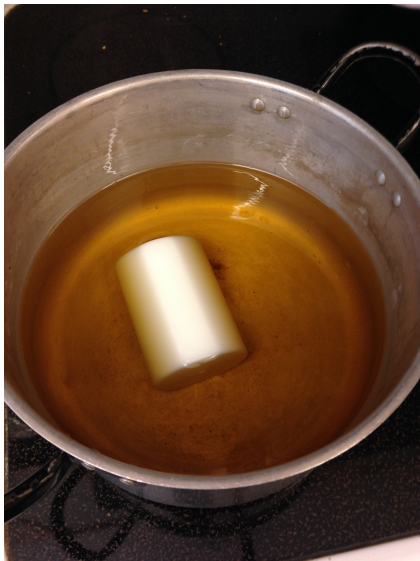
(a) The POM piston in an oil bath. Test to examine whether it would swell.
