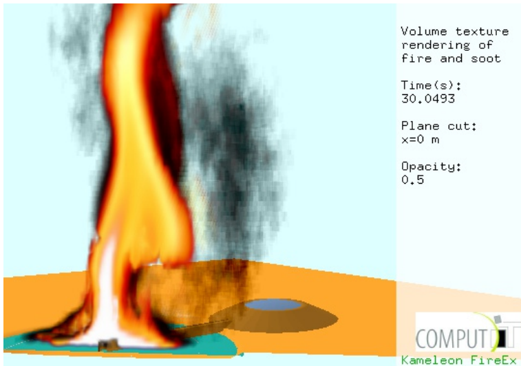
Figure 4.9: Volume texture rendering of sim16 at t \approx 30 s. Both the CAD import and flame and soot rendering was cut in the plane x = 0 m. Uncombusted fuel shows as white. Positive y -axis in the left horizontal direction, positive x -axis into the plane.
