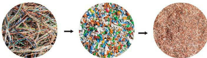
Figure 24 Cable separation process(20)
