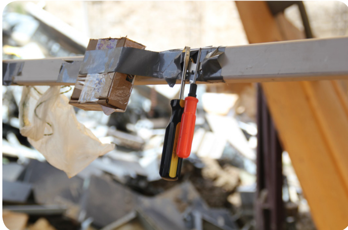
Figure 48 Prototype of tool holder made with magnets and duct tape
