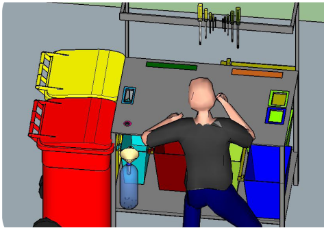
Figure 39 Dismantling table with colors marking each material hole
