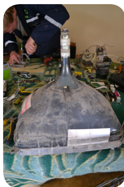
Figure 20 CRT element after stage 1 dismantling
