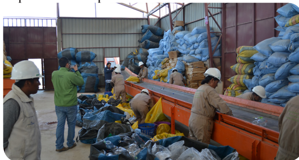
Figure 4 Classification plant at Alpacoma outside of La Paz. Workers separate the fractions manually
