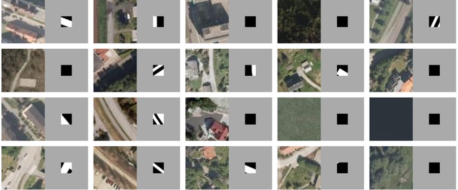
Figure 2.4: Aerial image and label examples from a patch dataset. The patches originate from the Norwegian Roads Dataset. Each label depicts the road ground truth from the center location of the aerial patch.
