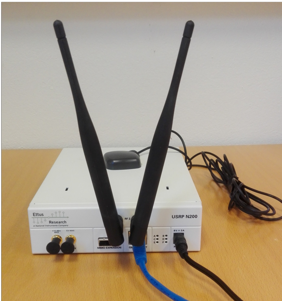
Figure 4.2: The N200 with GPS, VERT2450 antennas, Ethernet cable and power cable attached.
