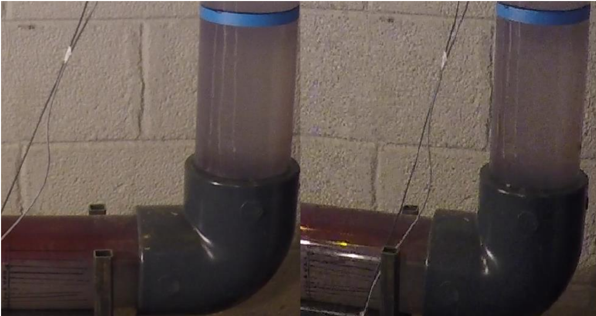
Figure 47 – Front height at displacement of second riser start ( 6\text{m}^3/\text{h} left and 30\text{m}^3/\text{h} right)
