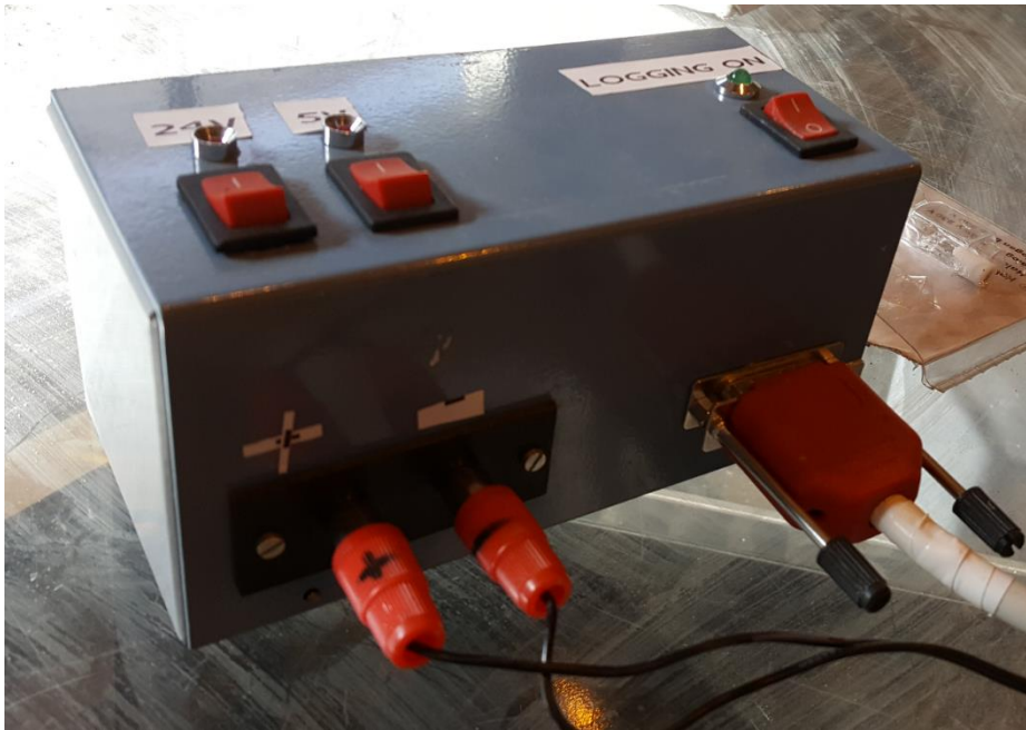
Figure 8 - External logging box
