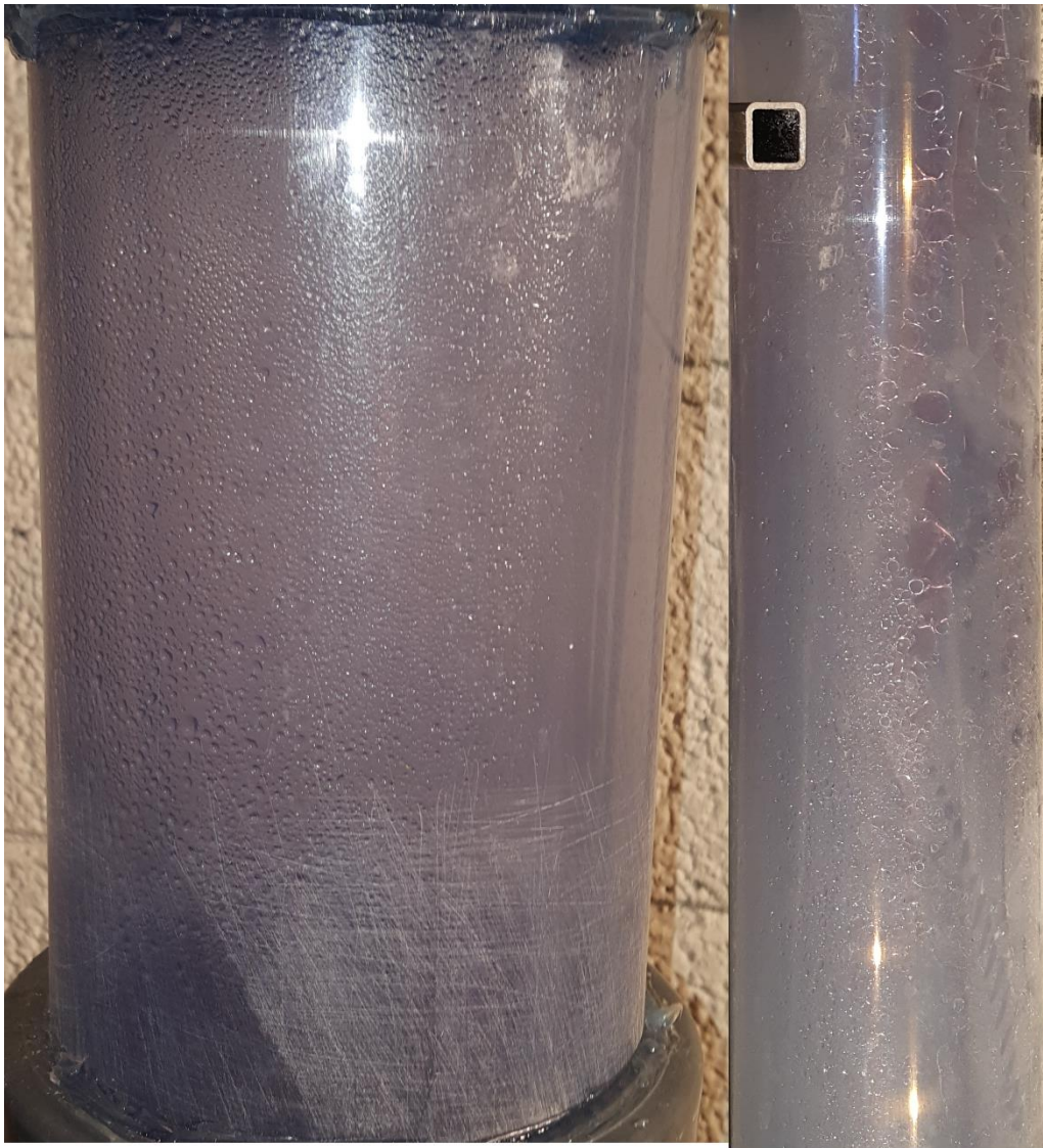
Figure 35 - Bubbles on wall of vertical section (left) and horizontal section (right)
