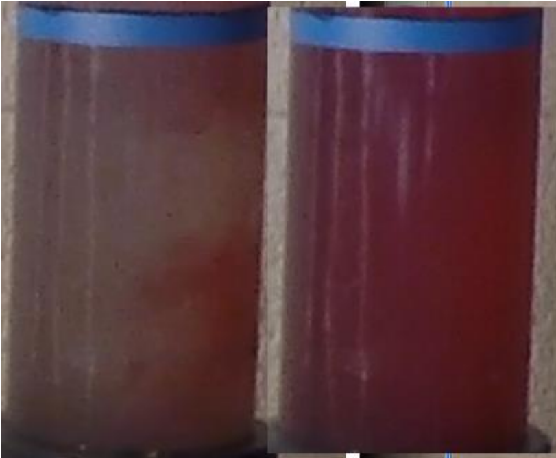
Figure 44 - Oil bubbles (left) and oil dominant (right) in bottom of second riser ( 8 \text{ m}^3/\text{h} )
