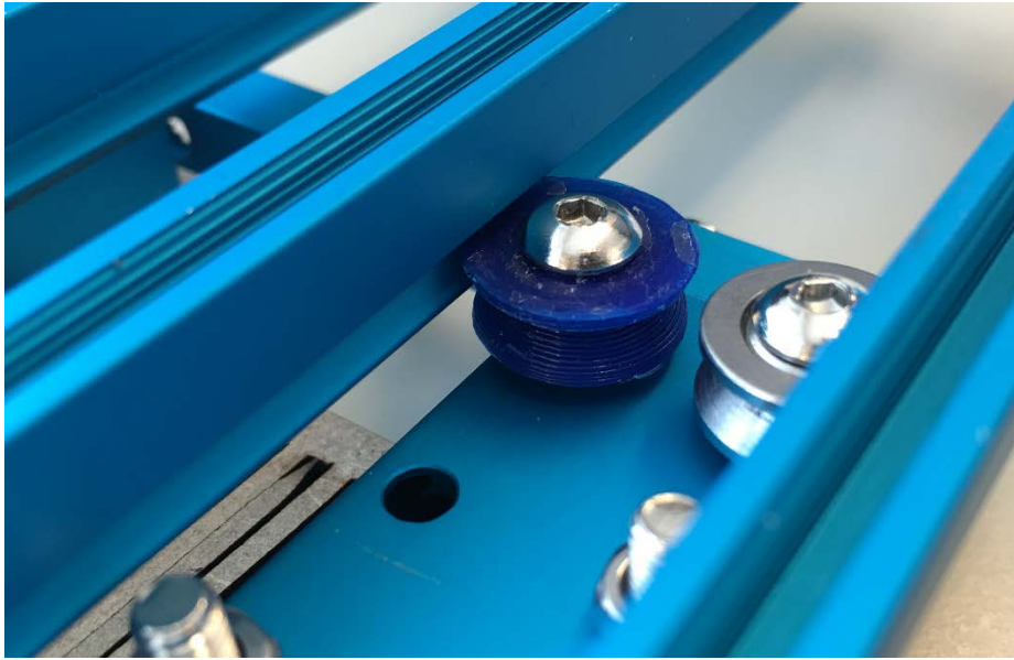
Figure 23 - 3D-printed bearings introduce more friction to rail mechanisms in all concepts.
