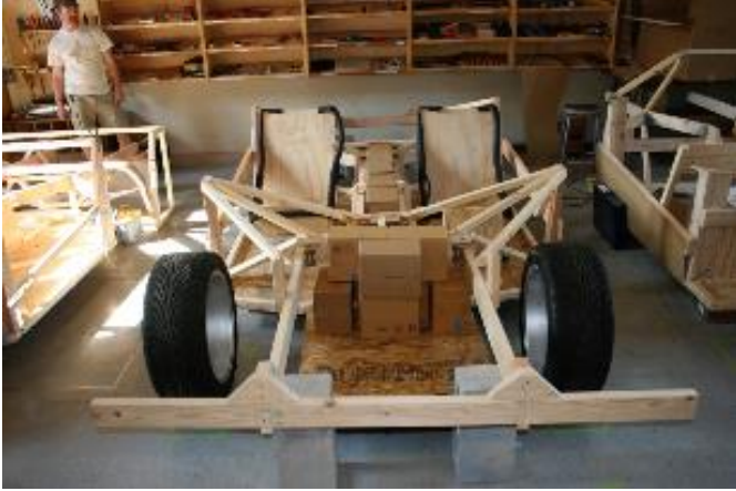
Fig. 4 An early wooden prototype of the ‘X1 Experimental Vehicle’.
