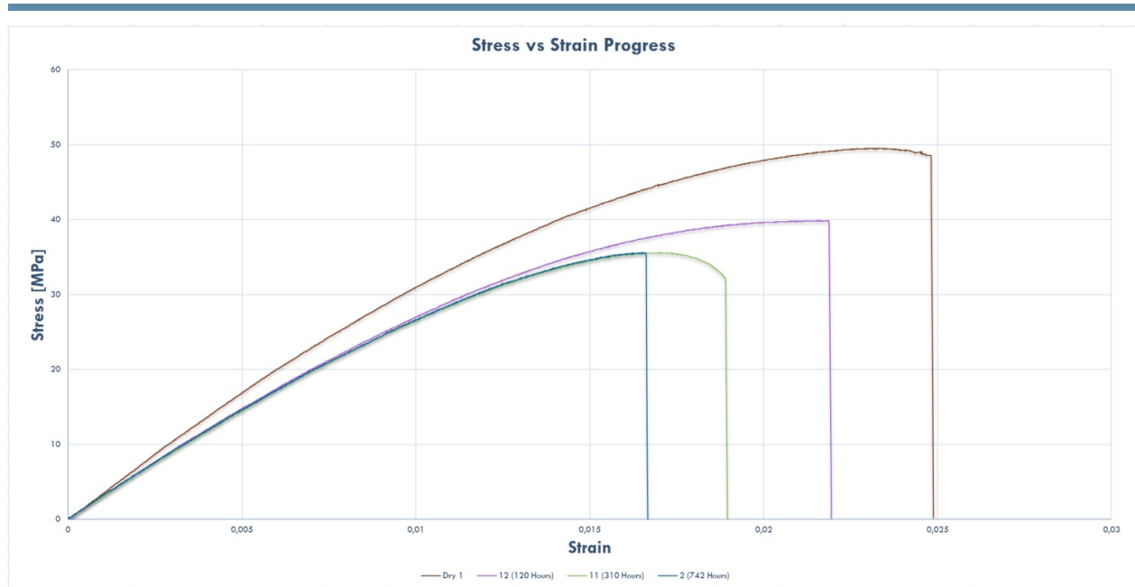
Figure 5.12: Representation of the changes in mechanical behaviour of Epoxy specimens during water diffusion process.
