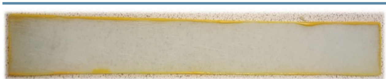
Figure 4.5: Coated specimen ready for labelling and water diffusion process.
