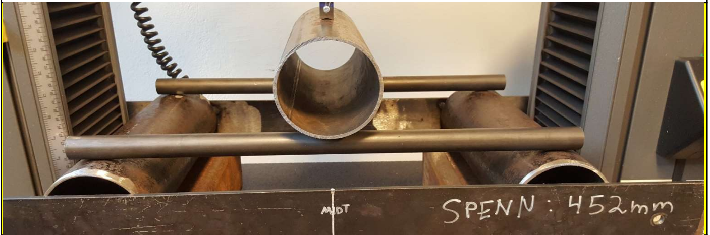
Figure 3: Test setup - Steel tube(s)
