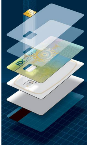
Figure 3.4: Smart card construction from [9]
