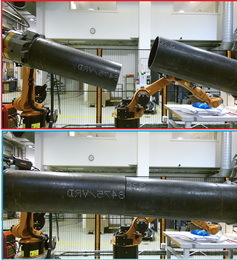
Figure 5.16: The upper part shows two tubes being tilted by the robots while the bottom figure shows the resulting fit-up using SAC-IA/ICP and Search Method.
