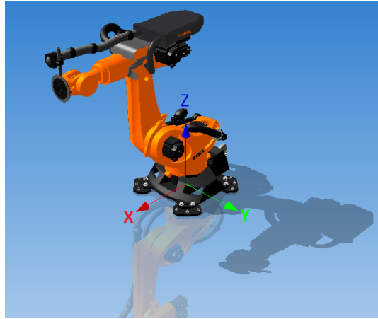
Figure 4.1: The coordinate system of the KUKA 120 R2500 robot.
