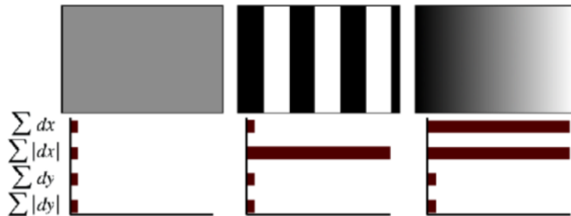
Figure 2.56: Illustration of the nature of a SURF descriptor. Left: A homogeneous region will make all values relatively low. Middle: Frequencies in x direction will make the value of \sum |d_x| high, but all others remain low. Right: In the case of a gradually increasing intensity in x direction, both values \sum d_x and \sum |d_x| are high. Image from Bay et al. (2008).
