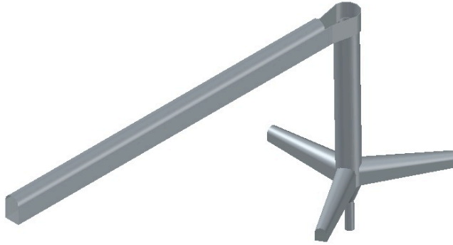
(a) The Krespa surge tank at the Obervermunt II PSP.
