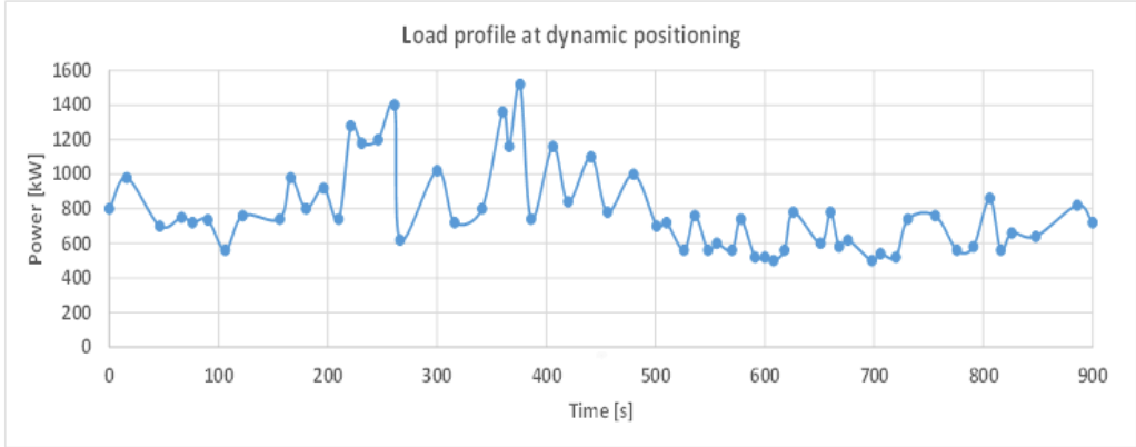
Figure 3.2: Total power supplied by two generator sets during dynamic positioning. This load profile is used for dimensioning of the HPS
