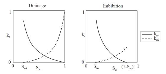
FIGURE 2.7: Typical relative permeability curves for water wet sandstone. (Zolotukhin and Ursin, 2000)
