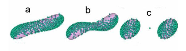
FIGURE 3.3: Breakup of oil droplets due to adsorption of nanoparticles. (Frijters et al., 2012)
