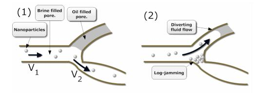
FIGURE 6.2: (1) Nanoparticles accumulate at the pore throat due to different flow velocities in the pore body and at the pore throat  $(V_1 \neq V_2)$ . (2) The pore throat will eventually be blocked, diverting fluid flow into other pores, which could be oil filled.
