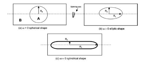
FIGURE 4.7: The spinning drop method. (Viades-Trejo and Gracia-Fadrique, 2007)
