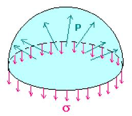
FIGURE 2.2: A droplet on surface. (Torsæter, 2012)
