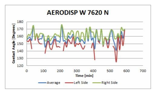
FIGURE B.3: Contact angle measurements of an oil droplet in AERODISP W  $7620~\mathrm{N}.$
