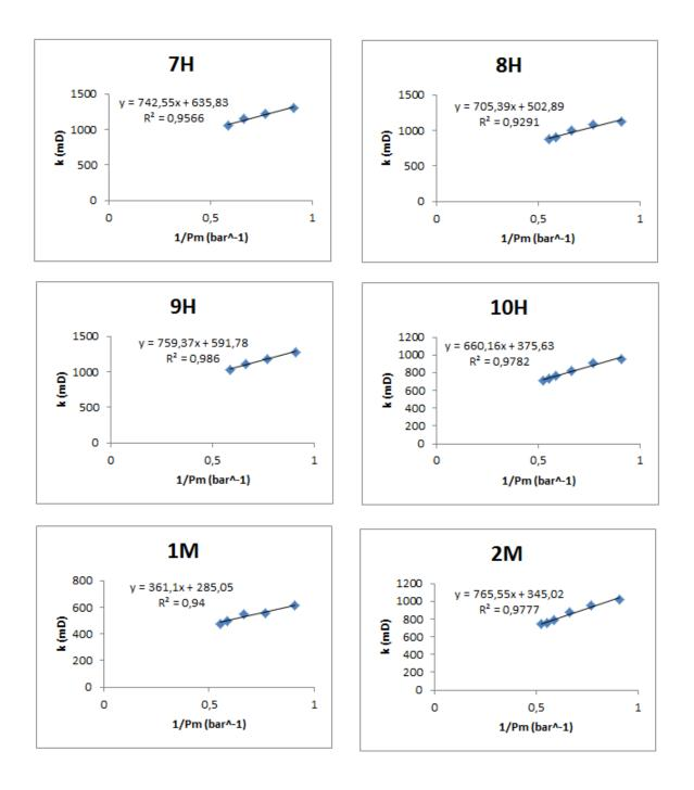
FIGURE A.2: Klinkenberg Plots for core 7H-10H and 1M-2M.
