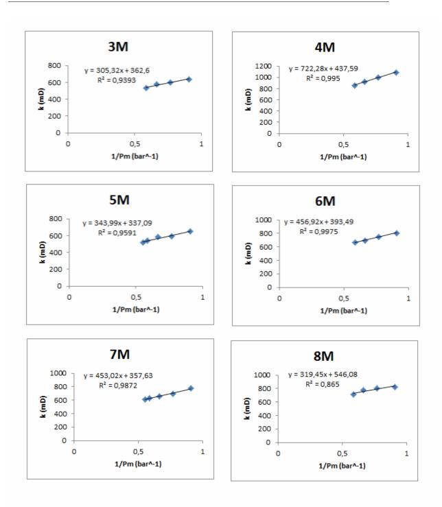
FIGURE A.3: Klinkenberg Plots for core 3M-8M.
