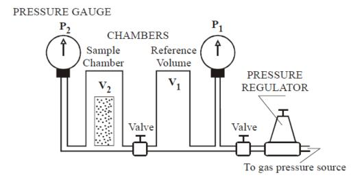
FIGURE 4.2: Helium porosimeter apparatus. (Torsæter and Abtahi, 2000)
