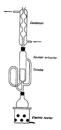
FIGURE 4.1: Soxhlet Extraction. (Torsæter and Abtahi, 2000)
