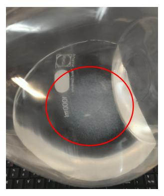
FIGURE 4.5: Precipitation of nanoparticles.
