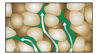
FIGURE 2.6: Connected pores gives permeability. (MPG Petroleum, 2003)
