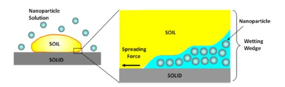
FIGURE 6.1: Spreading of nanoparticles on a solid surface. (Zhang et al., 2014)
