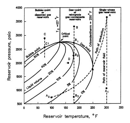
FIGURE 2.8: Two-phase diagram of reservoir fluids showing how they will vary with different pressure and temperature. (Whitson and Brulè, 2000)
