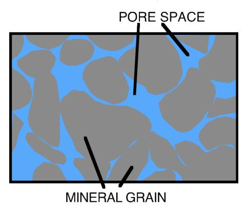
FIGURE 2.1: Pore space in a rock. (Wisconsin Geological Survey, 2010)
