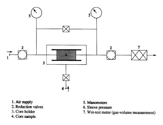
FIGURE 4.3: Constant Head Permeameter. (Torsæter and Abtahi, 2000)
