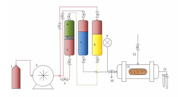
FIGURE 4.10: Experimental setup of the core flooding apparatus. 1) Exxsol D60 pump fluid, 2) pump, 3) valves, 4) Exxsol D60 displacing reservoir fluid, 5) piston to separate the oils, 6) crude oil, 7) NSB, 8) nanofluid, 9) pressure gauge, 10) bypass valve, 11) Hassler cell holder with core, 12) sleeve pressure, 13) effluent into test tubes. (Aurand et al., 2014)
