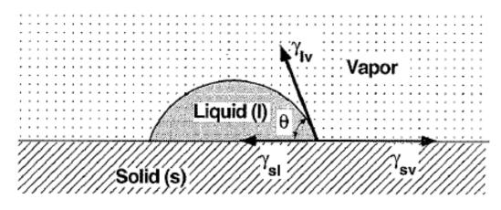
FIGURE 2.3: How the interfacial tensions works on a droplet/bubble. (Hiemenz and Rajagopalan, 1997)
