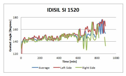
FIGURE B.7: Contact angle measurements of an oil droplet in IDISIL SI 1520.
