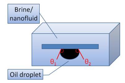
FIGURE 4.9: Imagining method for contact angle measurement.
