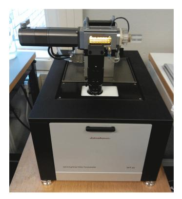
FIGURE 4.8: The spinning drop video tensiometer.
