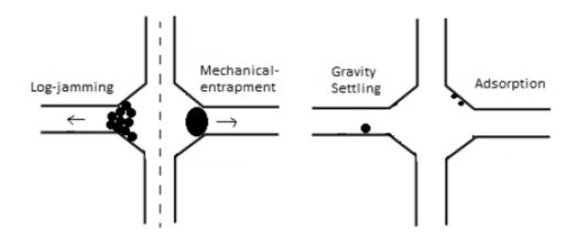
FIGURE 3.5: The four different mechanisms of retention. (Engeset, 2013)
