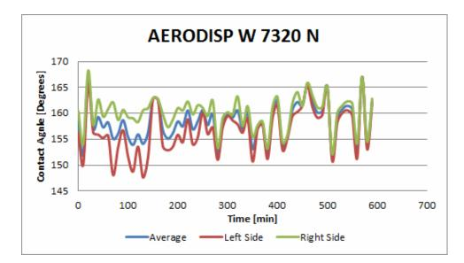
FIGURE B.5: Contact angle measurements of an oil droplet in AERODISP W  $7320~\mathrm{N}.$
