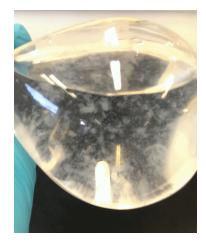
FIGURE 5.8: Fumed silica nanofluid after a week.
