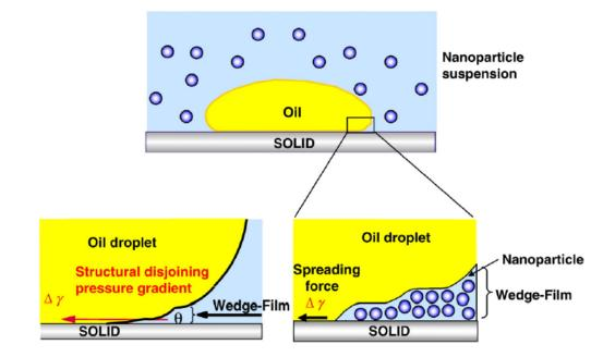
FIGURE 3.1: Nanoparticles establishing a wedge-film, resulting in a structural disjoining pressure. (Wasan et al., 2011)
