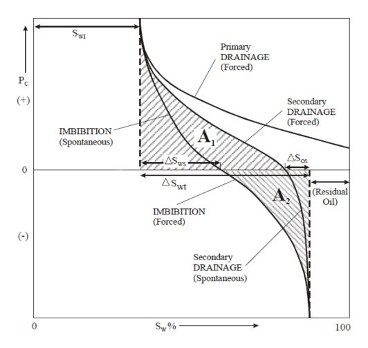
FIGURE 2.5: Typical capillary pressure curves. (Torsæter and Abtahi, 2000)
