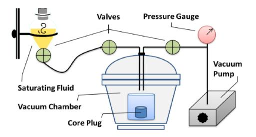
FIGURE 4.4: Vacuum pump setup. (Kaasa, 2013)
