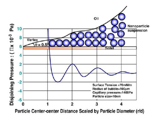
FIGURE 3.2: Disjoning pressure in the wedge structure. (Wasan and Nikolov, 2003)
