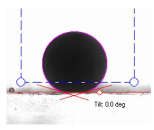
FIGURE B.1: The imaging method for measuring contact angle.
