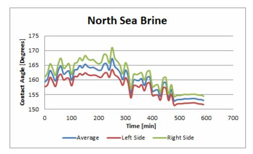
FIGURE B.2: Contact angle measurements of an oil droplet in North Sea Brine.
