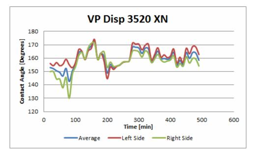
FIGURE B.4: Contact angle measurements of an oil droplet in VP Disp W 3520 N.
