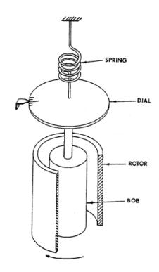
FIGURE 4.6: Rotating viscometer. (Torsæter and Abtahi, 2000)
