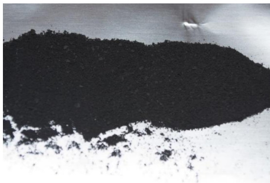
Figure 13 LMS and LFS powders after carbon coating and heat treatment
