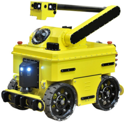
Figure 2.3: An early version of the maintenance robot "Sensabot", developed by National Robotic Engineering Center (NREC) (Image credits: NREC)
