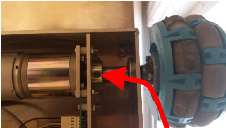
Figure C.1: The set screw which holds the wheel onto the motor drive shaft.
