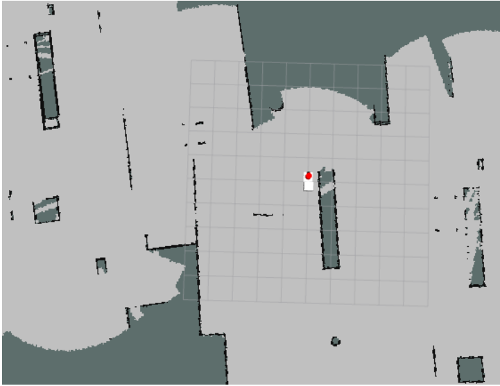
Figure 5.5: An example of incorrect map merging. This case occurred in the "Asphalt" world simulated in Gazebo.
