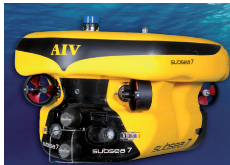
Figure 2.1: Subsea 7’s AIV. This is the first commercial autonomous inspection vehicle for subsea operations [pre]
